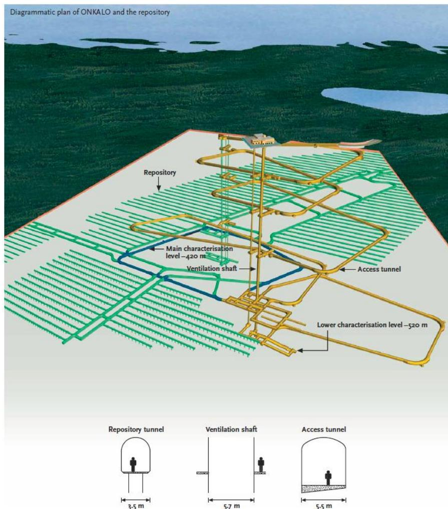
Fig. 2-1 Schematic illustration of ONKALO and disposal facilities (Posiva, 2006)
