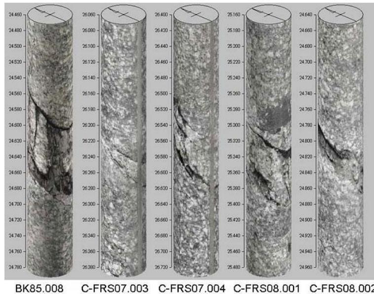
**Fig. 2-4 Sample images of target fractures taken by high resolution borehole camera (Nagra, 2013a)**
