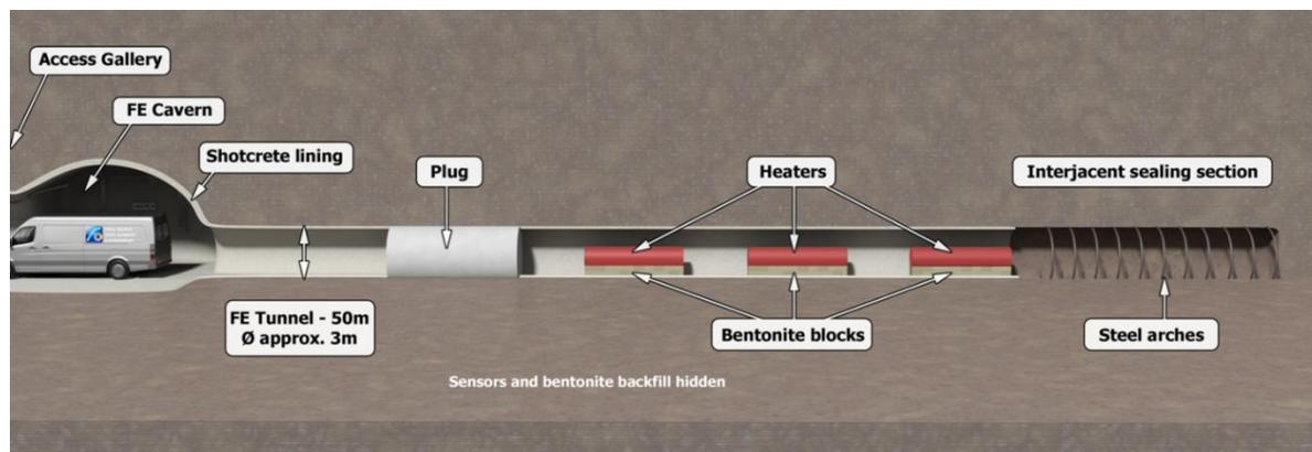
**Fig. 2-6 Schematic illustration of the FE layout (Vomvoris, et al., 2013)**
