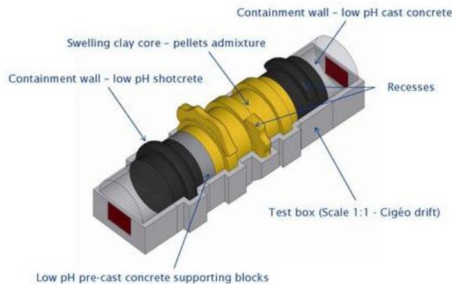
**Fig. 2-15 Layout of the FSS experiment (DOPAS, 2013)**
