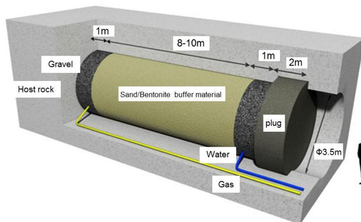
**Fig. 2-13 Schematic illustration of the GAST layout (modified from Nagra, 2013c)**
