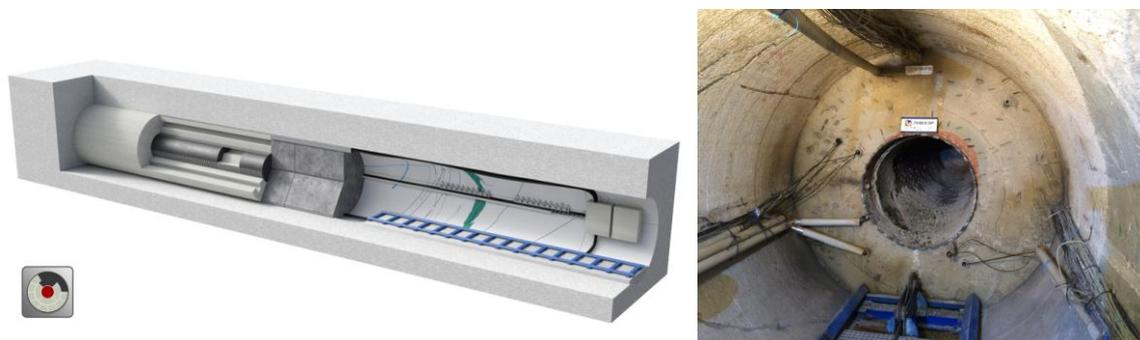
**Fig 2-7 Schematic illustration of the FEBEX experiment showing the heater and dummy canister surrounded by a bentonite block buffer and closed by a shotcrete plug (left); bentonite buffer with open heater section (right) (Nagra, 2015)**
