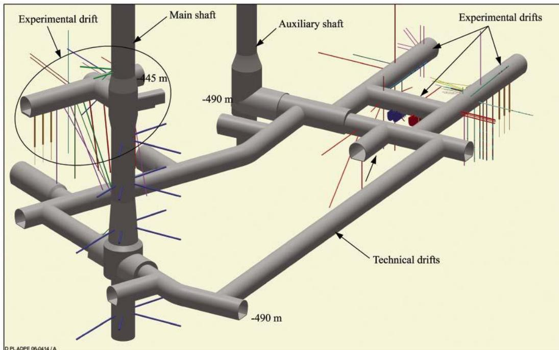
**Fig. 2-2 Layout plan of the Bure URL (Delay et al., 2011)**
