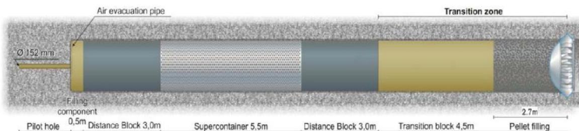
**Fig. 2-16 Schematic illustration of the MPT layout (SKB, 2013a)**
