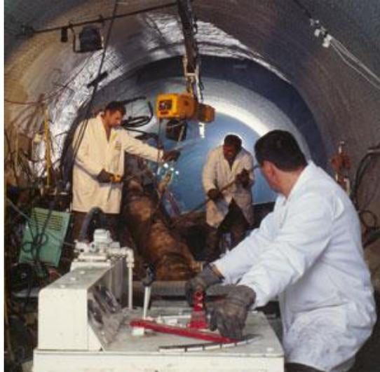
**Fig. 2-10 Overcoring the test intervals (Nagra, 2013b)**
