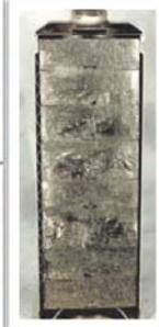
Metallic waste from reprocessing and metallic waste compacted into pellets, then placed in a stainless steel container
