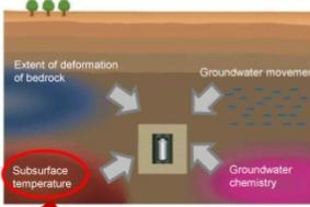
Due to the influence of the subsurface temperature and the decay heat of vitrified waste, if resultant temperature exceeds 100 °C over a long time period, it could adversely affect the buffer material.
