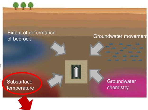
Due to the influence of the subsurface temperature and the decay heat of vitrified waste, if resultant temperature exceeds 100 °C over a long time period, it could adversely affect the buffer material.
