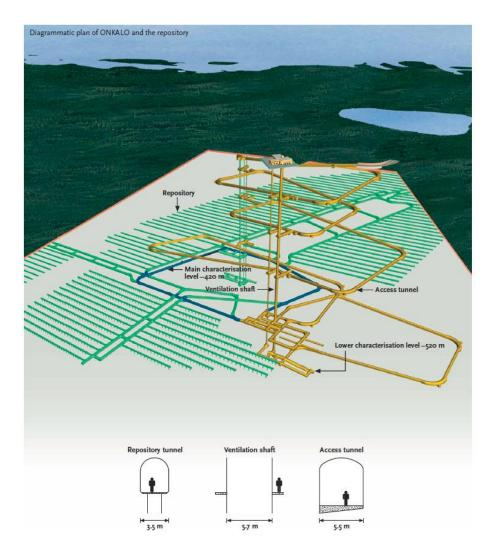
Fig. 2-1 Schematic illustration of ONKALO and disposal facilities (Posiva, 2006)
