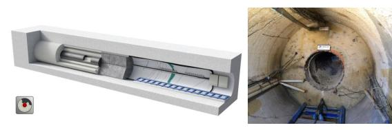
Fig 2-7 Schematic illustration of the FEBEX experiment showing the heater and dummy canister surrounded by a bentonite block buffer and closed by a shotcrete plug (left); bentonite buffer with open heater section (right) (Nagra, 2015)
