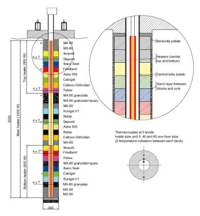
Fig. 2-9 Cross-section of a schematic illustration of the ABM test (Svensson, et al., 2011)
