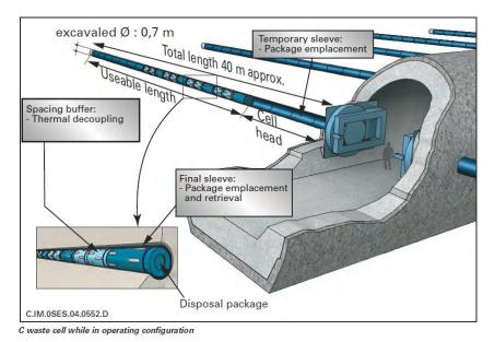
Fig. 2-5 Illustration of the concept for a C waste disposal cell (Andra, 2005)
