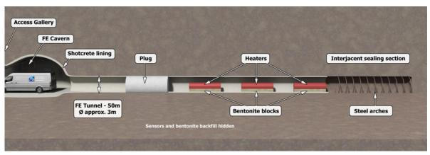
Fig. 2-6 Schematic illustration of the FE layout (Vomvoris, et al., 2013)
