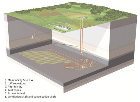
Fig. 2-3 Schematic illustration of the repository for SF/HLW/ILW (Nagra, 2014)
