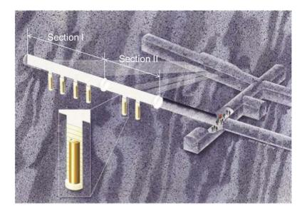
Fig. 2-11 Layout of the Prototype Repository (modified from SKB, 2012)
