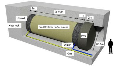
Fig. 2-13 Schematic illustration of the GAST layout (modified from Nagra, 2013c)
