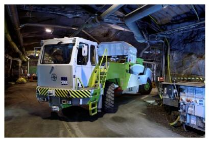
Fig. 2-17 Magne, the deposition machine (SKB, 2012)
