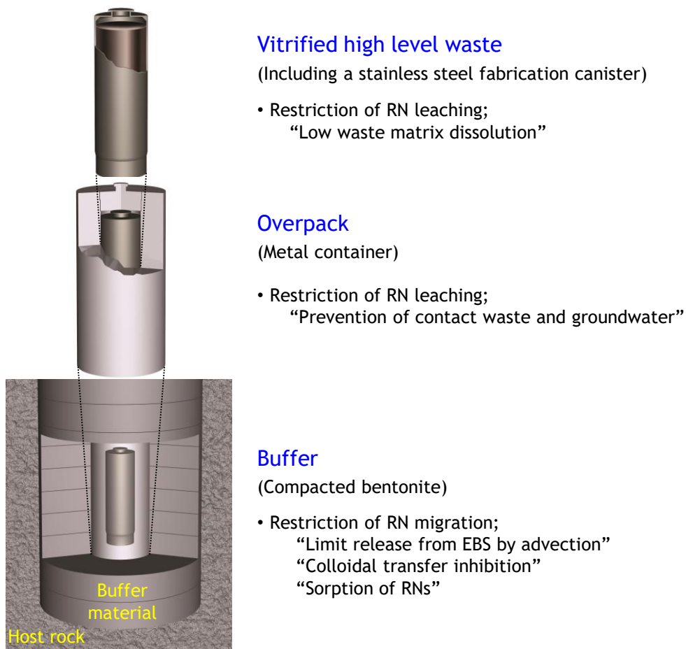
Figure 4.4-1 EBS for HLW and illustration of some associated safety functions (adapted from NUMO, 2004 [2])
