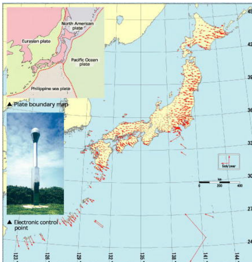
Figure 8-4: Vector map produced by analysis of horizontal crustal movement from April 2000 – March 2001 using the nationwide electronic control points (inset) established by GSI (fixed station: Ohgata, Japan Sea side of NE Japan). The map shows: a) relative crustal movements of the Japanese Islands where tectonic plates (inset) interact with each other; b) the different crustal movements of NE and SW Japan; c) the difference in crustal movements between SW Honshu and Shikoku along the Median Tectonic Line.
