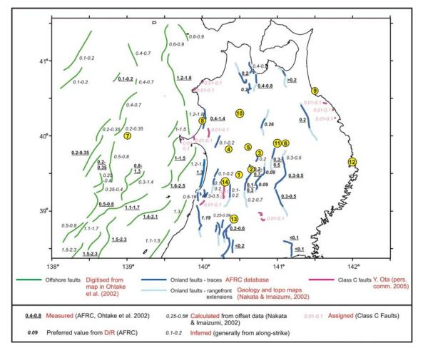
**Figure 3.1:** Active Fault source map for the Tohoku region. Fault sources are colour coded into groups relating to their data source, as summarised below the map. Vertical slip rates, in mm/year, are labelled and their data sources are also summarised below the map. The locations of the 14 example locations are shown in yellow.
