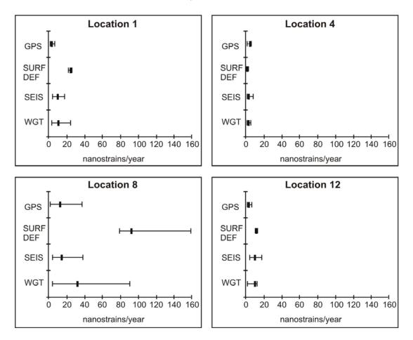
Figure 3.26: Strain rate uncertainties at four example locations. The weighted average rate (WGT) is derived from an equally weighted average of each of the GPS, surface deformation (SURF DEF), and seismicity (SEIS) values.
