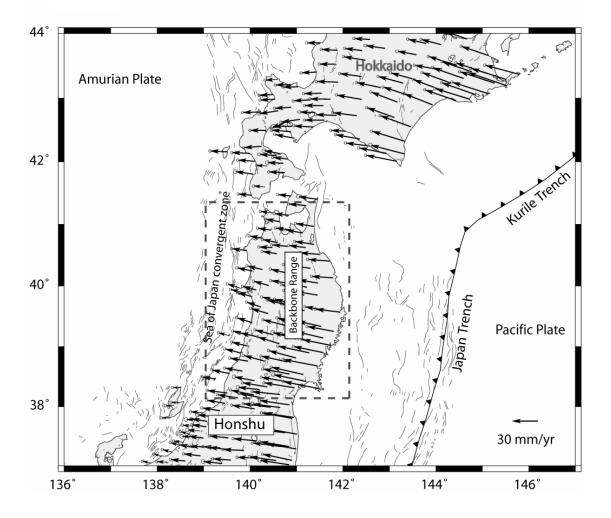
Figure 3.12: Tectonic setting and GPS velocity field in Northern Honshu (shown relative to a fixed Eurasian plate). Thinner black lines are active fault traces.
