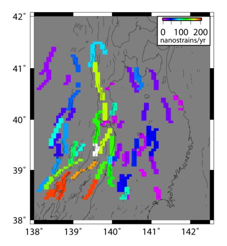
**Figure 3.4:** Strain map calculated for the active faults shown in Figure 3.1. The map is for the highest weighted realisation of the active fault branch of the logic tree shown in Figure 3.2
