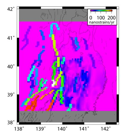
**Figure 3.9:** Surface deformation strain map. The strain values have been constructed from two datasets, active faults (onshore and offshore) shown in Figure 3.1, and tilt calculated from the uplift and subsidence contour map shown in Figure 3.3. The map shows the weighted average of all realisations of the logic tree shown in Figure 3.2.
