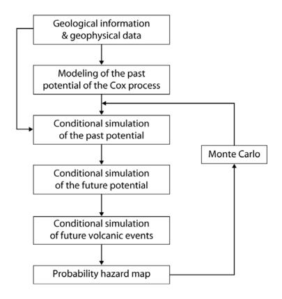
Figure 4.6. Flow chart of the Cox Process methodology for the estimation of volcanic hazard.
