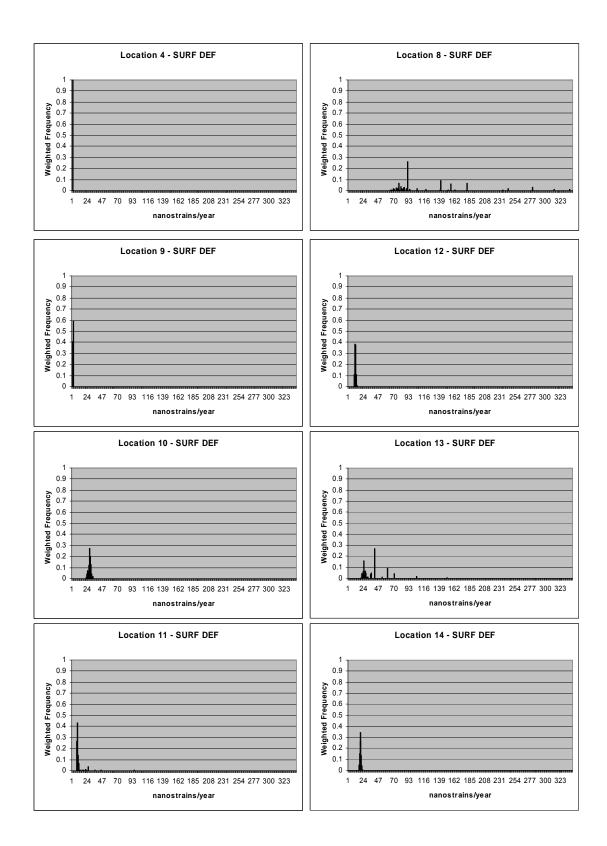
Figure 3.10 (continued from previous page): Strain histograms at 14 example locations from surface deformation.
