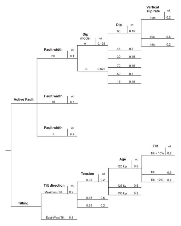
**Figure 3.2:** Summary logic tree for calculating strain rate from surface deformation. Note only one set of branches is shown. The weightings (wt) for the active fault model are as assigned by the expert panel, but the uplift mechanism model and the tilting model were assigned by the report authors.
