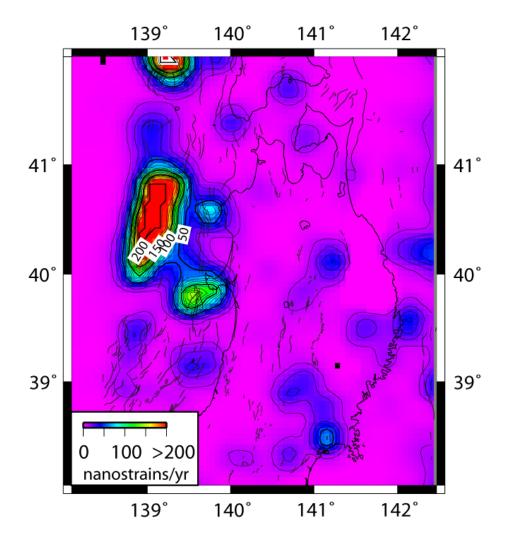
**Figure 3.22:** Seismicity strain map constructed from c. 400 year long record of historical and instrumental seismicity according to the logic tree shown in Figure 3.20. This plot is for the highest weighted realisation of the logic tree.
