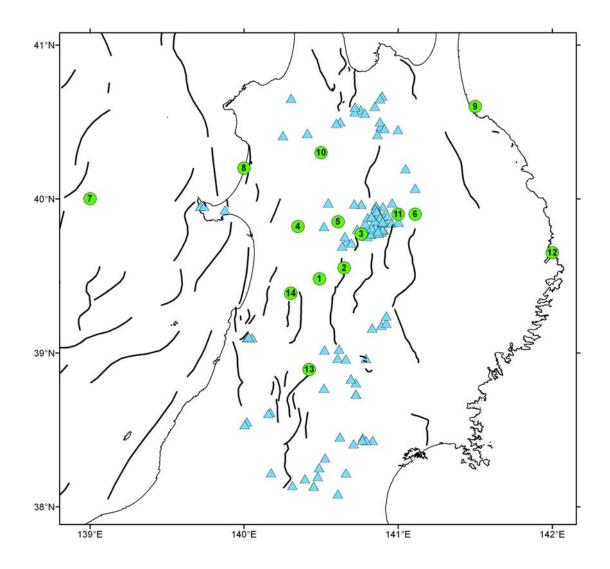
Figure 2.2: The fourteen example locations used in the Tohoku Case Study (green dots). Also shown are volcanic edifices (blue triangles) and active faults (bold, black lines). See Appendix for details.
