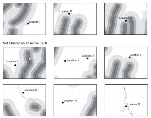
**Figure 3.5:** Locations of the 14 example locations with respect to active faults. The centreline of each active fault is shown as a black line, and the shaded buffer zones around each fault indicates the 5km, 10km and 20km wide process zones around each fault.
