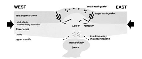
Figure 3.24: Schematic illustration of across-arc vertical cross-section of the crust and uppermost mantle, showing the characteristic shallow seismic activity and deformation of the crust beneath NE Japan (From Hasegawa, 2000).
