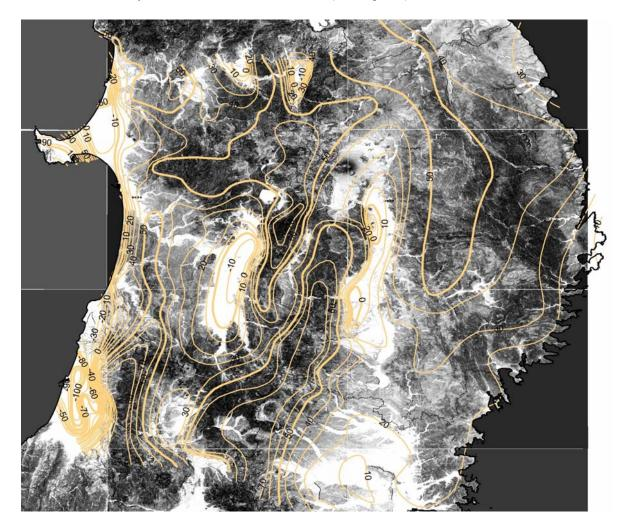
Figure 3.3: Uplift (and subsidence) contour map constructed from 125 ka fluvial and marine terraces. From Tajikara (2005).
