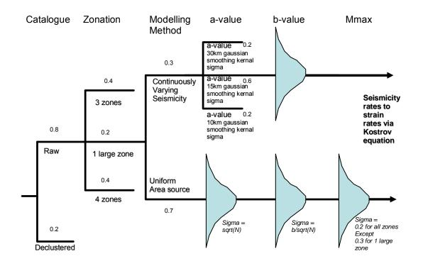
**Figure 3.20:** Logic tree structure developed for the seismicity strain model. This incorporated the expert elicitation meeting results of July 2005. The decimals shown are the weights assigned to each branch, and the schematic bell curve indicates that the parameter has a continuous normal distribution.
