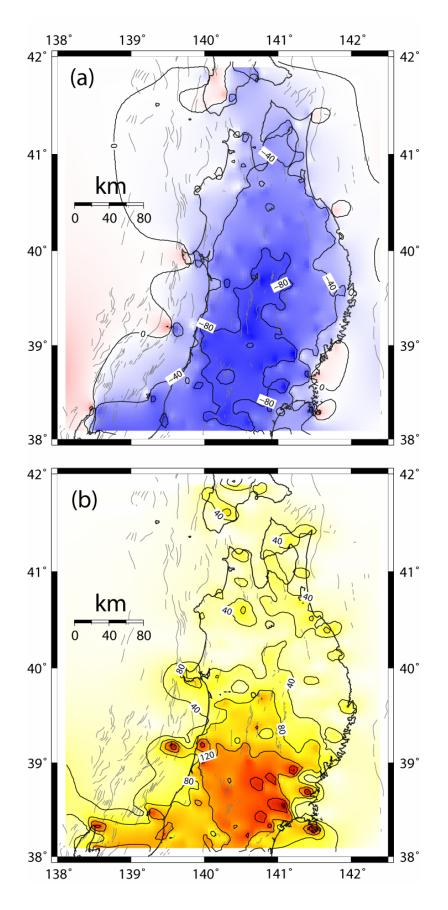
Figure 3.15: (a) areal and (b) shear strain rates from the raw GPS velocity field (see Figure 3.14; no elastic strains are removed) estimated using the Haines and Holt method. Strain rates shown in nanostrains/year.
