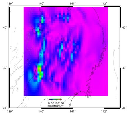
**Figure 3.7:** Strain map constructed for tilt calculated from the uplift and subsidence contour map in Figure 3.3. The map shows, for each grid square, the weighted average of all logic tree combinations shown in Figure 3.2. There are no tilt data offshore - the strain values in the offshore area are the result of edge effects of curve fitting to the tilt surface - see section 3.1.2.
