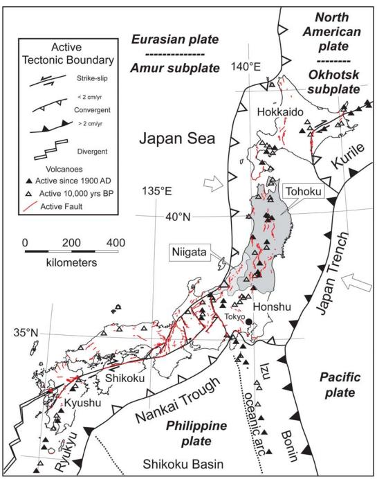
**Figure 2.1:** The principal plate tectonic features of Japan, showing the location of the Tohoku region of northern Honshu that forms the focus of this Case Study. The location of active faults and volcanoes that have been active in the last 10,000 years is also shown.
