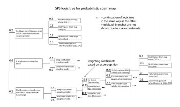
Figure 3.13: Logic Tree (with weightings shown) constructed by expert panel and used for probabilistic GPS strain map.
