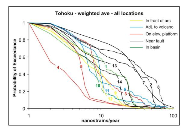
**Figure 3.28:** Plot of probability of exceedance of weighted average annual strain rates for 14 example locations. Example locations are approximately classified into tectonic domains of the study region. See Figure 3.1 for location of the 14 example locations
