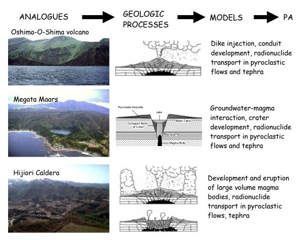
Figure 4.1: New volcanoes formed in the Tohoku region during the last 50 Ka represent a wide range of volcanic events in terms of magnitude and potential effects of volcanism. These different magnitudes and styles of volcanic activity should be reflected in performance assessment (PA) models of volcanism for a proposed HLW repository site. Volcanic hazard assessment is primarily concerned with determination of the likelihood of such events.
