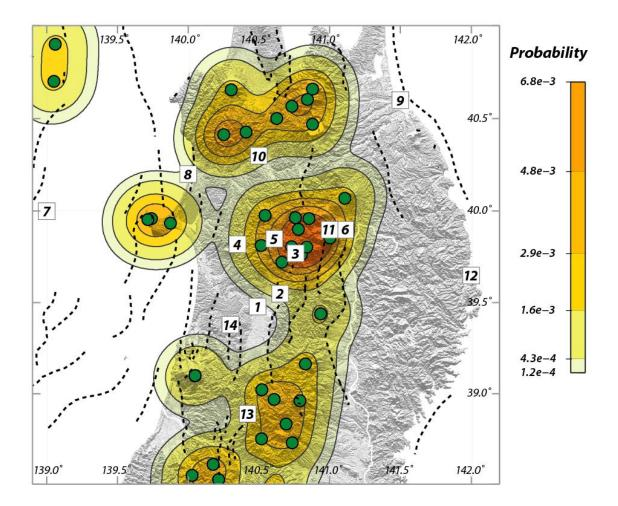
**Figure 4.11:** A clustered (LSCV) model of volcano spatial density calculated for the Tohoku region and showing the 14 example locations. This model best reflects a 'hot finger' model, with substantial variation in spatial density along the volcanic arc. Spatial density is shown as the probability of a new volcano forming within a 25 km<sup>2</sup> area during 100,000 yr. Darker orange colours indicate a higher spatial density, and therefore higher probability of a volcanic event.
