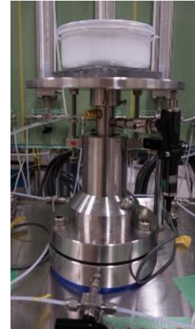
Figure 4-28 Swelling deformation test apparatus
