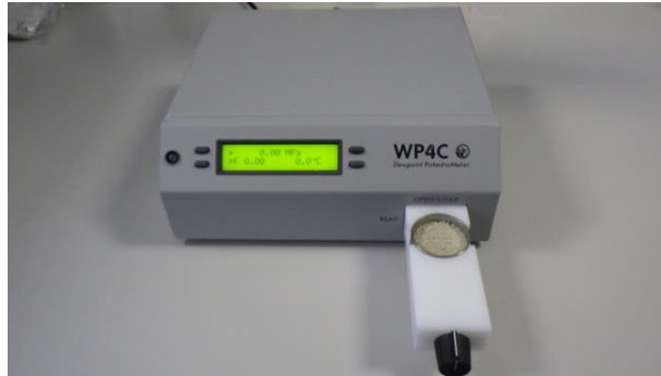
Figure 4-68 Measurement by chilled mirror hygrometer
