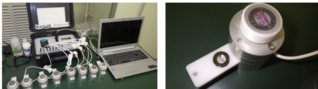
Figure 4-67 Measurement by thermocouple psychrometer
