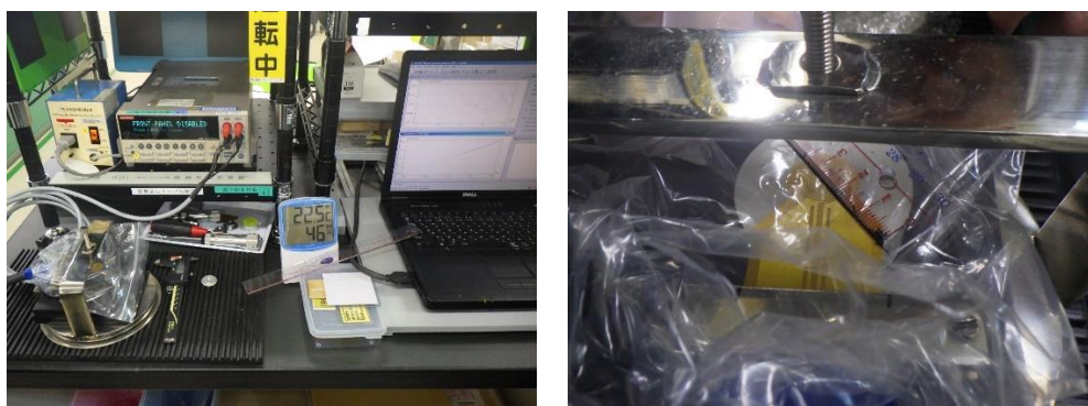
Figure 4-79 Measuring status of thermophysical property by HD method
