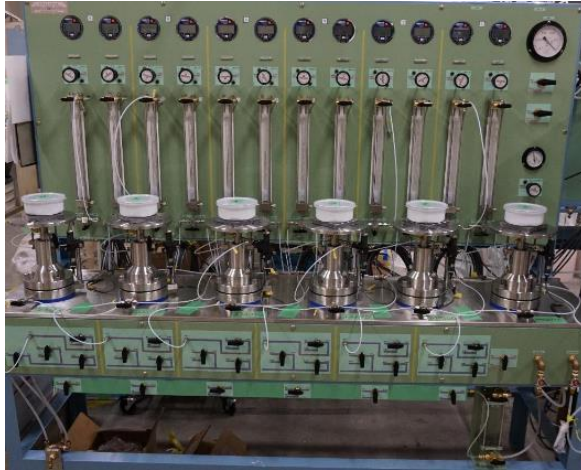
Figure 4-27 Whole view of apparatus for swelling deformation test equipped a measurement system of permeability
