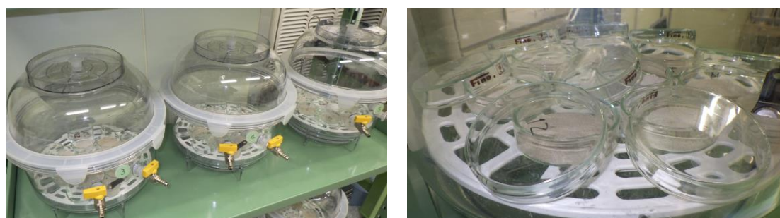
Figure 4-66 Measurement by vapor pressure method
