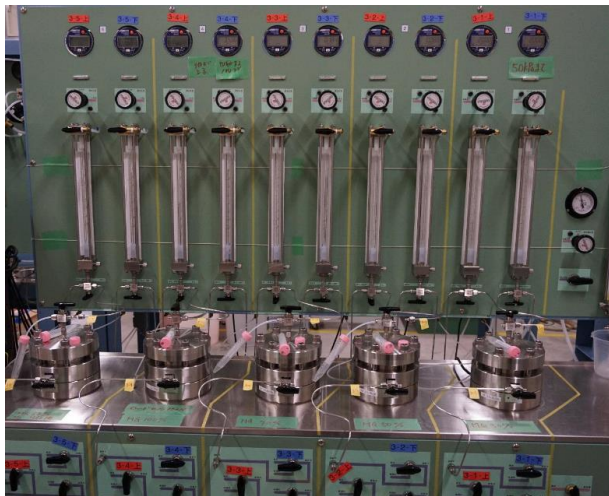
Figure 4-11 Whole view of apparatus for the permeability-swelling pressure test
